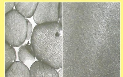
EPS (18 kg/m<sup>3</sup>) Finnfoam (32 kg/m<sup>3</sup>)
