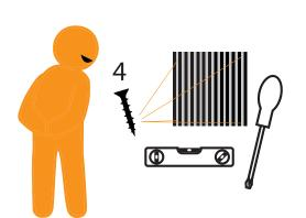
Use screws to install the acoustic panels on a wall or ceiling. You need 4 screws for each panel.
