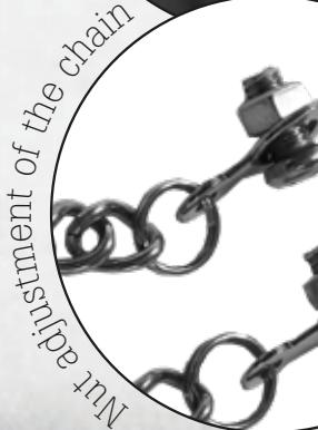
Fasten the chain to the holes in the side of the Grill-Smoking Oven between the upper and the lower part. Adjust the nut in the chain so that the chain can move freely, and fasten the chain from the inside of the Grill-Smoking Oven with a flange nut in the upper and lower part. Tighten the screws with the spanner.
