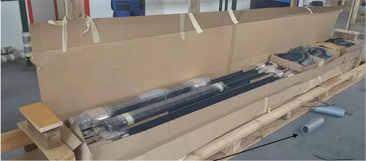
Please keep the grey sponges for later use as a padding underneath the frame / sections / sliding door during the assembly to avoid damages
